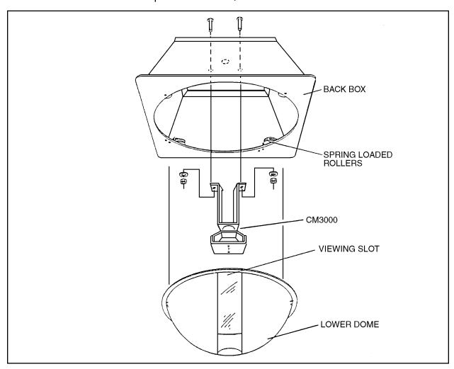
Figure 1. Installing the CM3000 in the SB3-1 Enclosure
